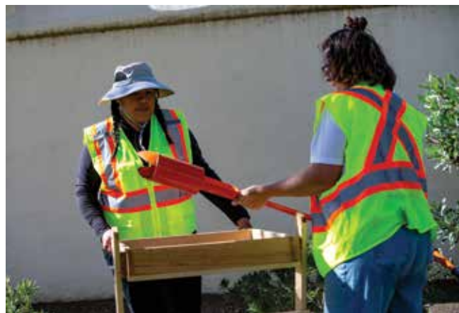
Yeneth Renteria holds the screen while Karisa Smathers unloads a soil sample from the auger.
